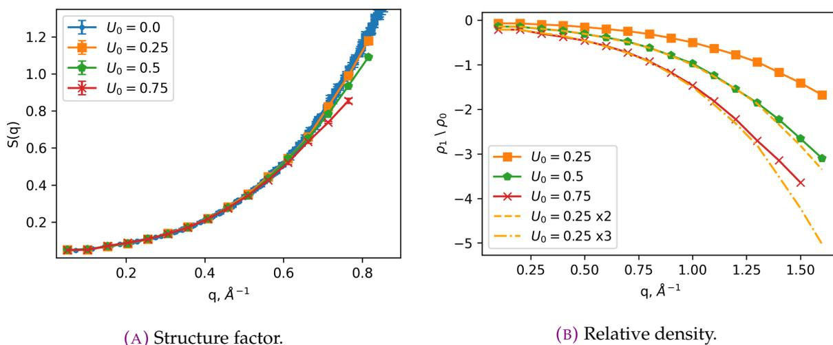
**FIGURE 4.8:** (A) Structure factor as a function of wave-vector  $\mathbf{q}$  calculated in the presence of an external field. (B) Relative density obtained in the external potential. In both cases,  $U_0$  is the amplitude of the force field,  $\times 2$ ,  $\times 3$  means that the results for  $U_0 = 0.25$  kcal/(mol $\cdot\text{\AA}$ ) were multiplied twice or three times correspondingly to check the linearity of the response. Results shown for the GL bead.
