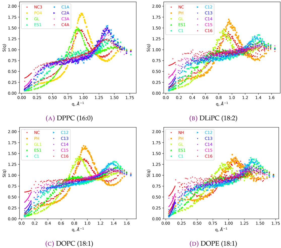
**FIGURE C.3:** A full structure factor dependence on the bead type for available model lipids: DPPC, DLiPC, DOPC, DOPE. Systems of 512 lipids and 8192 water beads at  $T=298$  K and  $P=1$  atm.
