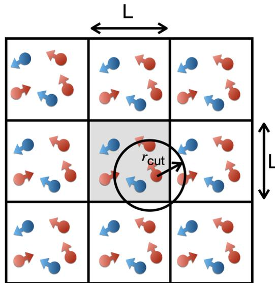
**FIGURE 3.1:** Schematic illustration of the periodic boundary conditions. The unit cell is marked gray and has size  $L$ , it consists of red and blue particles,  $r_{\text{cut}}$  is the maximum interaction distance. Images of the simulation cell are shown around the initial unit cell.
