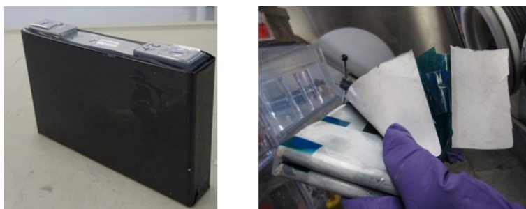
Figure 88. Illustration of the Samsung PHEV 37 Ah and its connected rolls found inside
