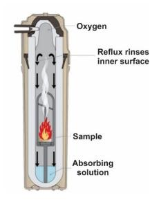
Figure 3. Commercial system used for the decomposition of samples by MIC, demonstrating the burning of a sample and the reflux of the absorbing solution promoted by microwave heating (adapted from Microwave Reaction System for Sample Preparation, Anton Paar, http://anton-paar.com).
