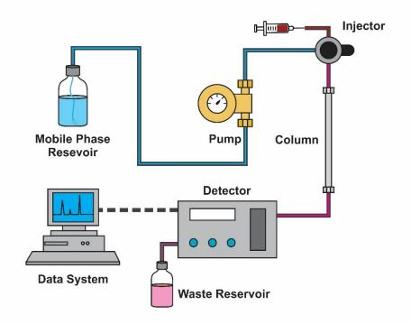
Figure 1. Basic components of a HPLC system.
