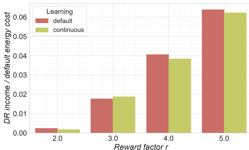
Figure 6.5: DR participation income relative to the baseline energy cost. Initial training on Nov. 2002, and retraining every month. The continuous learning case income is compared to the default one, where a whole winter season dataset is used for learning before integrating the DR program. DR participation during Dec. 2002 - March 2003.
