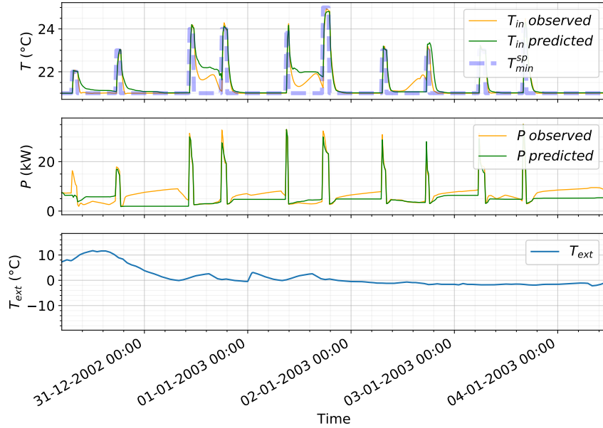
Figure 4.22: 24-hour ahead forecasting results. Auto-regressive RF estimators for indoor temperature: T_{in,t} \approx f_{RF}(X_t, X_{t-1}, T_{in,t-1}) , X = (T_{sp}^{min}, T_{ext}, \Phi_{irr})^T , and power consumption: P_t \approx f_{RF}(X_t, X_{t-1}, P_{t-1}) , X = (T_{in}, T_{sp}^{min}, T_{ext}, \Phi_{irr})^T . Validation on IDA ICE building with simulated preheating operations.
