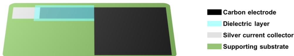
**Figure V-7** – Illustrative representation of the complete screen-printed gas diffusion electrode containing a silver current collector, a dielectric layer in blue, and the carbon electrode. GDL design type **B** is represented.
