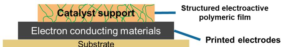
**Figure I-19** – Second layer of the fully printed H<sup>+</sup>/CO<sub>2</sub> reduction electrode: a catalyst-supporting layer based on a structured electroactive polymeric film.
