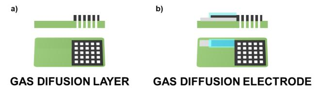
Figure V-3 – Schematic representation of the screen-printed gas diffusion layer (a) and gas diffusion electrode (b).
