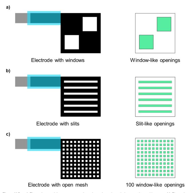
**Figure V-5 – a)** Electrode containing two square-shaped openings, *i.e.*, windows, on its working area. **b)** Electrode containing six rectangular openings, *i.e.*, slits, on its working area. **c)** Electrode with an open-mesh design containing one hundred window-like openings.
