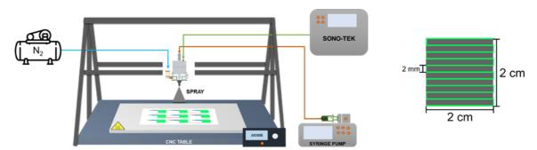
**Figure I-16 – Left:** Ultrasonic spray setup including a CNC table; heating bed, compressed N<sub>2</sub> feed, ink feed provided by a syringe pump; the Sono-Tek fluxing system, air, and flux controller, and ultrasonic nozzle. **Right:** Spray path for catalyst deposition (green line) over 4 cm<sup>2</sup> printed gas diffusion layer (GDL).
