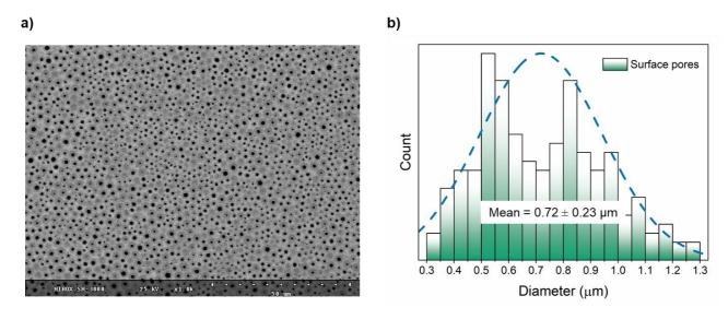
**Figure II-20 – a)** SEM top view and **b)** pore size distribution of pre-doped P(S-*stat*-BuA)-*b*-TANI film cast on Nafion HP with DCM. The film was green with a white surface.
