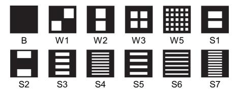
**Figure V-30 –** Selected printed GDL designs to study GDL's design influence on the electrochemical performance of the printed GDL electrodes.
