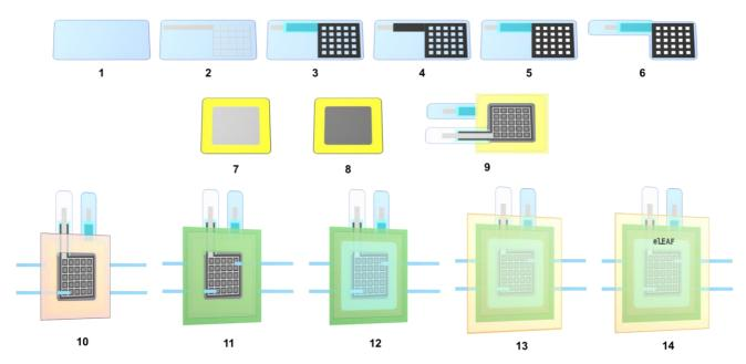
**Figure V-61 –** Methodology for the preparation of printed GDL electrodes (top row) and membrane electrode assembly for e<sup>-</sup>LEAF (middle row) and assembly of the e<sup>-</sup>LEAF cell.
