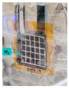
**Figure V-60 –** Pictures of the anode (left) and cathode (right) of  $e^{-}LEAF$  in operation demonstrating the production of  $O_2$  and  $H_2$  by electrolysis powered by the photovoltaic cell.
