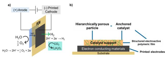
Figure I-17 – Conceptual illustration of a membrane electrode assembly (MEA) containing a printed cathode for H<sup>+</sup>/CO<sub>2</sub> reduction (a) and a cross-sectional illustration of the architecture of the fully printed cathode.
