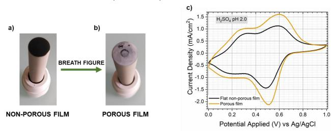
**Figure II-22 –** Pictures of H<sub>2</sub>SO<sub>4</sub>-doped the, **a)**, non-porous and, **b)**, porous films of P(S-*stat*-BuA)-*b*-TANI characterized electrochemically, and, **c)**, cyclic voltammetry results obtained in H<sub>2</sub>SO<sub>4</sub> (pH 2) as the electrolyte at room temperature.
