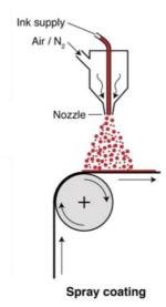
Figure I-15 - Schematic illustration of spray coating. Adapted from [214].
