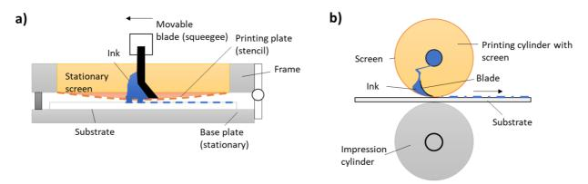
Figure I-14 – Schematic representation of a) flat-to-flat and b) round-to-round screen-printing techniques. Adapted from [191]
