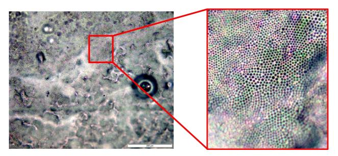
**Figure II-23 –** Optical micrographs of the porous film H<sub>2</sub>SO<sub>4</sub>-doped P(S-*stat*-BuA)-*b*-TANI cast on top of a Pt electrode for electrochemical characterization.
