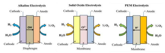
Figure I-3 - Schematic illustrations of AWE, SOE, and PEM electrolysis. Adapted from [52].
