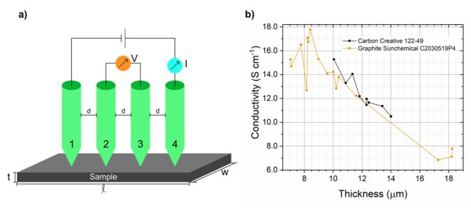
**Figure V-14 – a)** Four-Point Probe system where t, w, and  $\ell$  represent the thickness, width, and length of the sample, respectively, and d is the distance between probes. **b)** Measured conductivity of screen-printed electrodes from different inks.
