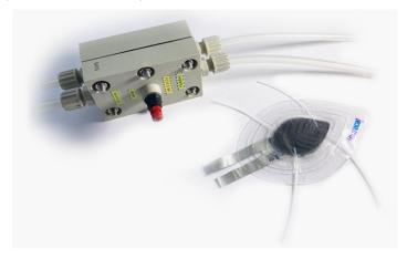
Figure V-51 - Picture of commercially available electrolyser cell and e<sup>-</sup>LEAF.
