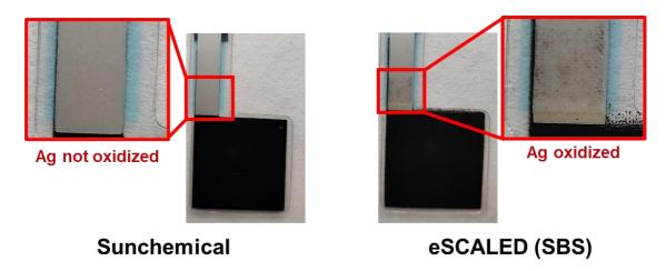
**Figure V-45 –** Pictures of Sunchemical and eSCALED (SBS) printed GDL electrodes after being submitted to the SRS experiments to assess the ECSA of each electrode. The oxidized Ag is observed by the appearance of dark grey spots at the current collectors.
