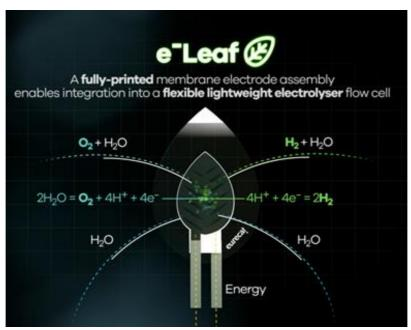
Figure V-50 - Schematic representation of the e<sup>-</sup>LEAF concept: a fully printed MEA in a flexible lightweight cell.
