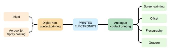
**Figure I-12 –** Printing technologies for printed electronics manufacturing.
