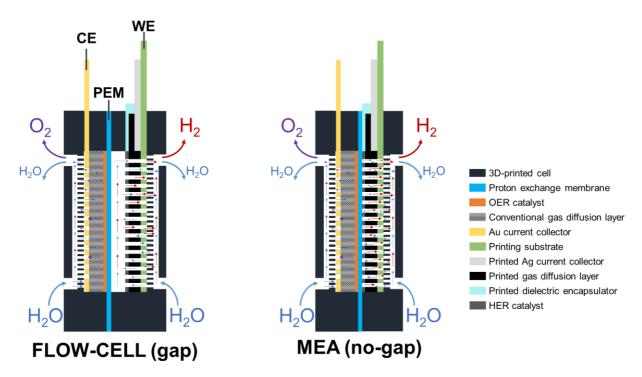
**Figure V-35 –** Cross-sectional schematic view of the flow-cell (gap) and membrane electrode assembly (MEA, no-gap) configurations with an integrated screen-printed electrode to host the HER studied inside a 3D-printed electrolyzer cell.
