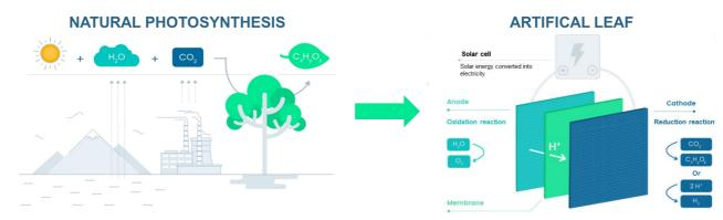
Figure I-4 – eSCALED's proposed artificial leaf architecture. Visit http://escaled-project.eu/ for more details.
