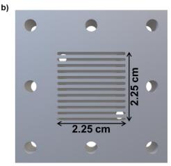
**Figure V-4** – End-plate design of the conventional electrolyzer cell available for the testing of the MEAs: **a)** external side with flow inlet and outlet, **b)** inner side of the end plate with 2.25 x 2.25 cm² flow distribution area.
