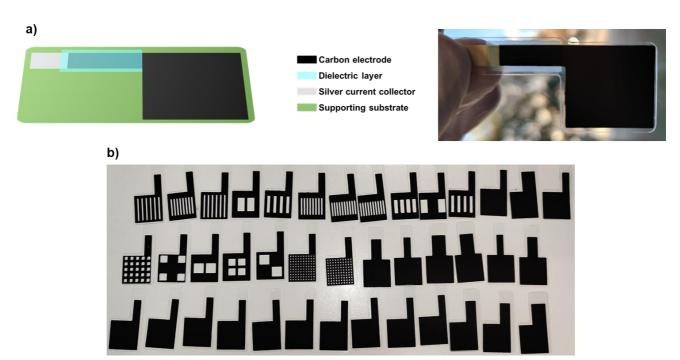
Figure V-11 – Screen-printed GDL electrode (design type B) schematic representation (a) and picture of a prepared sample on polymer foil (b). Printed GDL samples prepared in all building blocks designed and proposed.
