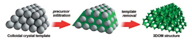
**Figure IV-1** – Steps of colloidal crystal templating for the fabrication of a three-dimensionally ordered macroporous (3DOM) structure. Adapted from [22].
