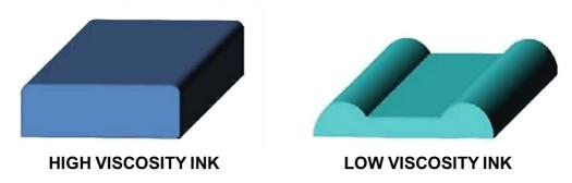
Figure V-42 - Typical cross-section pattern from printed inks with high and low viscosity. Adapted from. [54]
