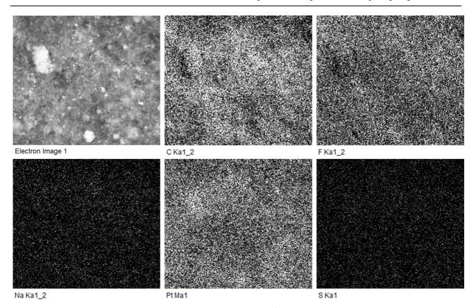
Figure V-20 - SEM-EDS elemental mapping of Pt-coated (0.17 mg/cm<sup>2</sup>) printed GDL electrode.
