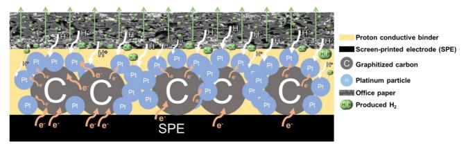
**Figure V-46 –** Cross-section of the printed GDL electrode on a porous supporting electrode. The produced  $H_2$  is expected to diffuse through the porous supporting substrate.
