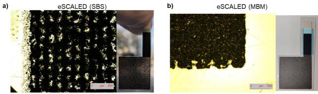
**Figure V-40 –** Micrographs and pictures from the screen- printed GDL electrodes from **a)** Graphite eSCALED (SBS).and **b)** Graphite eSCALED (MBM).
