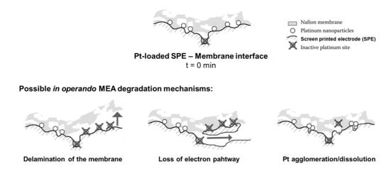
**Figure V-39 –** Cross-sectional perspective of the Pt-loaded printed GDL – membrane interface in MEA configuration and possible *in operando* degradation of mechanisms of the MEA. Adapted from [51].
