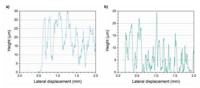
**Figure V-41 –** Height profiles of the screen-printed GDLs from **a)** Graphite eSCALED (MBM) and **b)** Graphite eSCALED (SBS) (three wet on wet layers).
