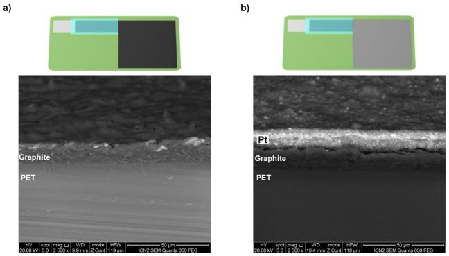
Figure V-19 - Cross-sectional SEM images of a) bare printed GDL electrodes with type B design and b) Pt-coated (0.17 mg/cm²) SPE.
