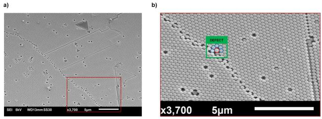
**Figure IV-6 – a)** Top view SEM images of the obtained PS templates (sample 9). **b)** Defect detected in the PSs template (sample 9) attributed to the presence of a PS sphere larger (red circle) than the neighbor PS spheres (blue circles).
