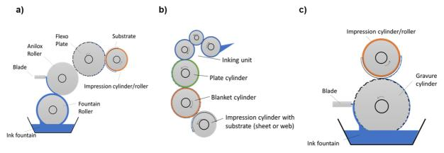
Figure I-13 – Analogue printing methods: a) flexography, b) offset, and c) gravure printing. Adapted from [191].
