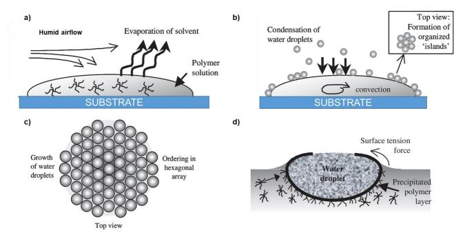
**Figure II-15 –** Formation of honeycomb-structured porous films. **a)** Evaporation of the solvent in the polymer solution; **b)** condensation of water droplets; **c)** hexagonally packed water droplets on the surface of the solution; **d)** precipitation of the polymer on the interface. Adapted from [33].
