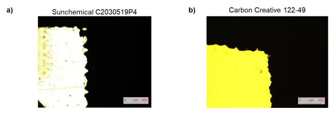
**Figure V-12 –** Micrographs and pictures from screen-printed electrodes from **a)** Graphite Sunchemical C2030519P4 and **b)** Carbon Creative 122-49.
