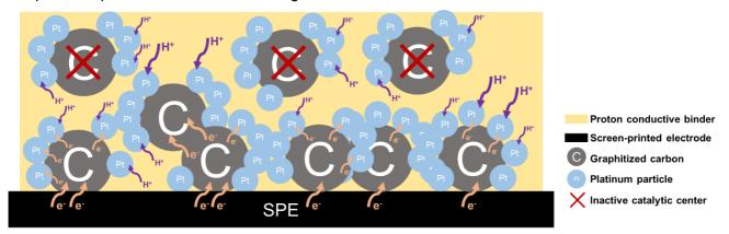
**Figure V-22 –** Cross-sectional illustration of proton and electron transport paths on a Pt-coated printed GDL electrodes. In the case of the present thesis, the proton conductive binder used was Nafion.
