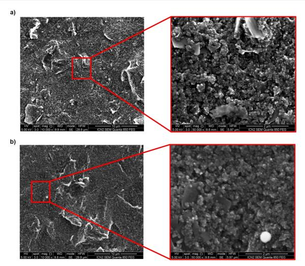
**Figure V-29 -** SEM images from the top view of bare printed GDL electrode **a)** before and **b)** after being submitted to electrochemical characterization (applied potentials between 0 and -2.1 V (vs Ag/AgCl) in PBS pH 7 at 40 °C).
