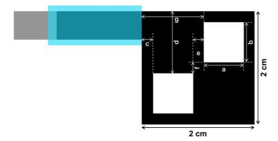
Figure V-8 - Parametrization of dimensions design of screen-printed gas diffusion layers. GDL design type W1 is represented.
