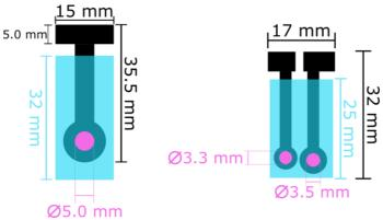
**Figure V-63 –** Screen-printed electrode designs. Black and blue colors represent the carbon and insulating layers, respectively. The pink color represents the working area of the electrodes. Adapted from <sup>[65]</sup>.
