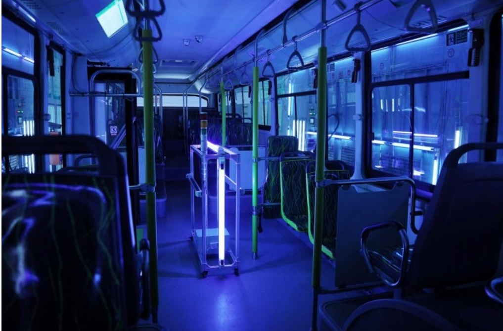
Figure 6: UV lamp used to disinfect a bus during Covid-19 pandemic.
