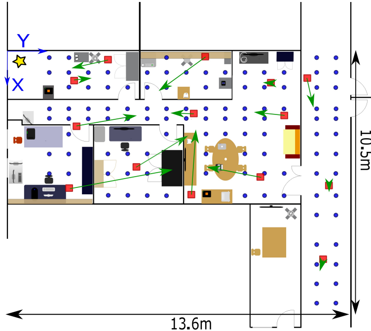
Figure 6.5 – Mean localization error per testing location (green arrow) in meters plotted in the experiment area (DelFin). Yellow star is the gateway.
