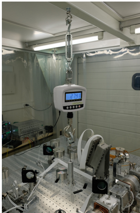
Figure 5.5.: Lifting and weighing of SQB1 at LAPP.
