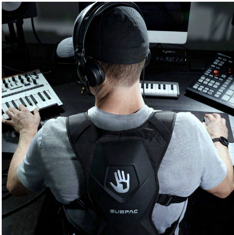
Figure 13: SUBPAC, M2X version (Crofts, 2018). The wearable haptic device transmits bass vibrations to the user's back, in time with their auditory content. Along with music, it is also advertised for use in gaming, virtual reality, and home cinema experiences. SUBPAC was also imagined as an inclusive device for individuals with hearing impairments, so that they can have an immersive experience of sound via the sense of touch.
