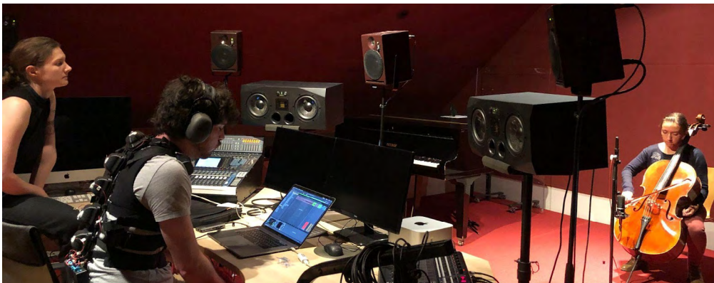
Figure 76: During a test session, we worked with a cellist to explore the potential of the sensory experience: the listener, wearing the multimodal harness, feels and hears the vibrations of the instrument in real time.
