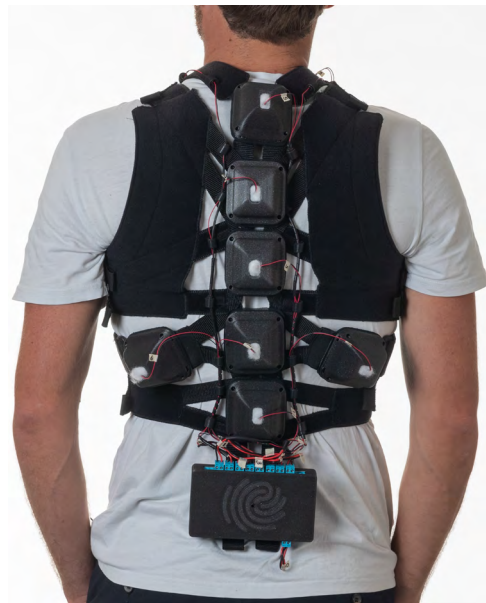
Fig. 1. The multimodal harness elicits both auditory and tactile perception, via extra-tympanic (bone) conduction and vibrotactile stimulation of the skin surface. The wearable device was designed with adjustable velcro straps, which suit users with waist dimensions between 64 and 90 cm. Photo credit: Véronique Huyghe.
