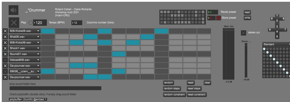
Figure 72: The Drummer interface seen in the Max environment. The sequencer tracks each correspond to one actuator position on the harness. Above the sequencer, there is a preset grid for saving specific drumming patterns.
