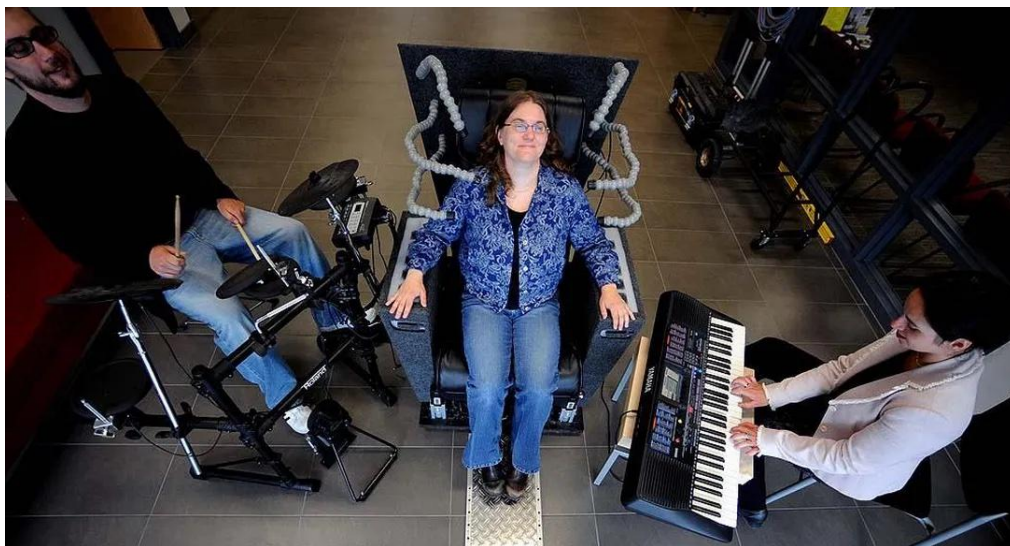
Figure 16: The EmotiChair is a vibrating chair that transmits vibrations along the user’s arms, back, and seat according to the frequencies of the auditory input. In the photo, it is in use by Ellen Hibbard, who is deaf. After using the EmotiChair, she said that she “never really thought about ‘bad’ and ‘good’ feelings with vibrations,” ... “This experience has helped [her] to understand why hearing people have strong feelings when they listen to music” (Black, 2008).
