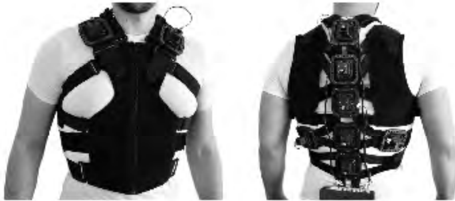
Fig. 1. The multimodal harness. Nine voice-coil motors (Atronika HapCoil) are integrated in the wearable structure inside hard plastic modules on the clavicles, spine and ribs. The velcro straps tighten the modules' contact against the body, whose vibrations penetrate the body to elicit ETC sound perception, and stimulate the skin for tactile sensations. Users receive earplugs and a noise-reducing headset (3M Peltor XEA) in order to protect them from all external noises created by the actuators and ensure they hear only via ETC.
