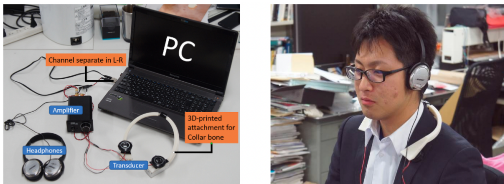
Figure 11: The CollarBeat (left: technical setup, right: in use). The authors designed and 3D-printed a neck-worn device with two voice-coil vibrotactile motors situated on the user's collarbones. The contact between the user's body and the device is ensured via 100g weights on both ends of the wearable device. Images extracted from Sakuragi et al. (2015).
