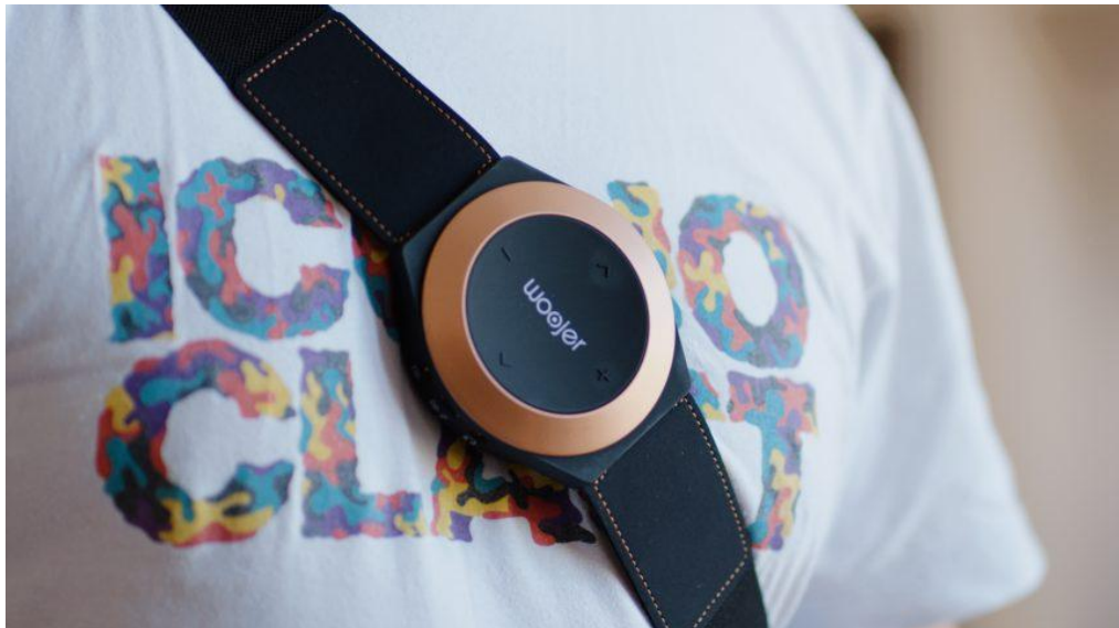
Figure 15: The Woojer Strap Edge integrates one vibratory motor, encased in the central unit of the strap. Its form means it is adjustable to virtually all body sizes. It is portable and simple in design in comparison to other vest-style audio-tactile devices. Image retrieved from: https://www.woojer.com/products/strap-3
