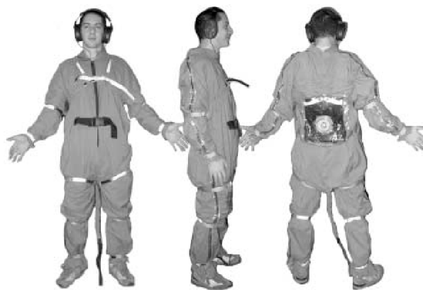
Figure 10: The Vibrotactile composition suit, a full-body audio-tactile wearable system designed by Gunther and O’Modhrain (2003) that integrates thirteen vibrotactile voice-coil motors. To create tactile effects perceived simultaneously with music, the authors approached the composition process from a multimodal standpoint: the tactile effects and auditory music were designed in parallel. The auditory effects were perceived via the attached headset, seen in the photo. Image extracted from Gunther and O’Modhrain (2003).
