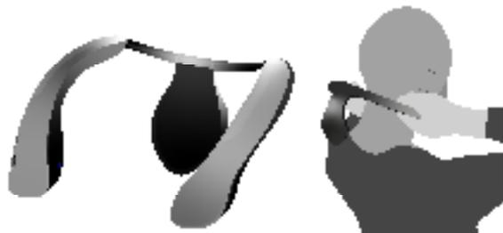
**Fig. 5.** The product design artifact. A preliminary illustration of the future *Ryann*<sup>TM</sup> device, designed for tactile augmentation of listening. The device integrates three positions of vibrotactile stimulation on the upper neck and clavicles.
