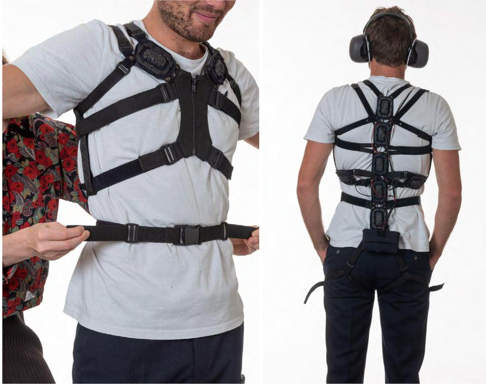
Figure 37: Photos of the MH.1 audio-tactile wearable device. Users wear the device on top of their clothing, ideally with no more than one layer to reduce vibratory signal attenuation. To maximize the device adjustability to different body types while maintaining consistent pressure of the vibratory modules against the body, there are seven points of adjustment on either side of the body (14 total velcro adjustments). (Photo credit: Véronique Huyghe).
