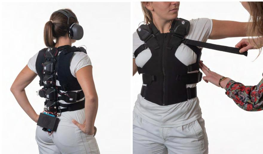
Figure 39: The second iteration of the multimodal harness (MH.2). The main design changes for this version of the wearable audio-tactile device are resumed in section 3.2.2. (Photo credit: Véronique Huyghe).
