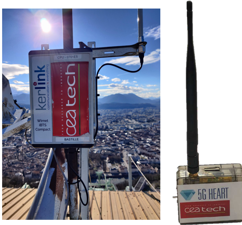
(a) Gateway BS_3 which is installed on the roof near the cable car station at Bastille, (b) Tag which was used to collect the data
