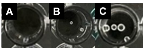
Figure 4.8. Catalase mimics of Pt-based NanoZymes after 5 minutes. Control experiment, H 2 O 2 +Buffer (A). PtSeeds catalase-mimics, H 2 O 2 +PtSeeds+Buffer; [Pt] = 2.8 \mu M (B). LN/Pt catalase-mimics, H 2 O 2 +LN/Pt+Buffer; [Pt] = 2.8 \mu M; [LiNbO 3 ] = 14.5 \mu M (C). For all the samples, the measurements were performed in the presence of H 2 O 2 (29.7 mM) at pH 4 (acetate buffer) and 37°C. All the concentrations are in the reaction well.
