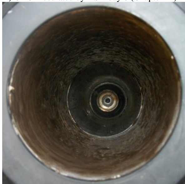
Figure 29: photos of the experimental segment-pipes just after the application of the centrifugated activated-sludge for CAC lining, (A) corresponding to the experiences realized with AS 1 presented in the chapter III, (B) corresponding to the experiences realized with AS 2 presented in the chapter VI.
