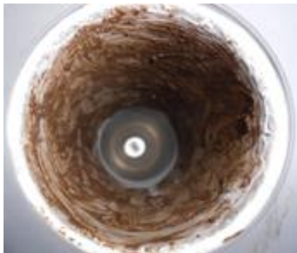
Figure 29: photos of the experimental segment-pipes just after the application of the centrifugated activated-sludge for CAC lining, (A) corresponding to the experiences realized with AS 1 presented in the chapter III, (B) corresponding to the experiences realized with AS 2 presented in the chapter VI.
