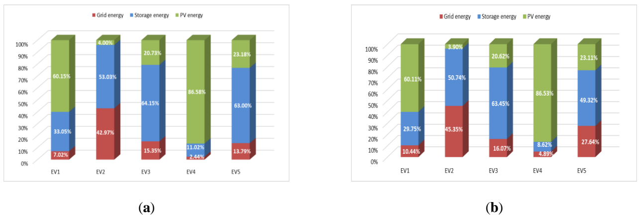
Figure 94: EV energy distribution for “real-time exp” (a) without opt and (b) with opt—experimental test 5.
