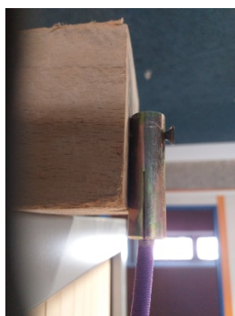
Figure 3.10: Hinge and target used for the experiment - Cable with targets mounted on
