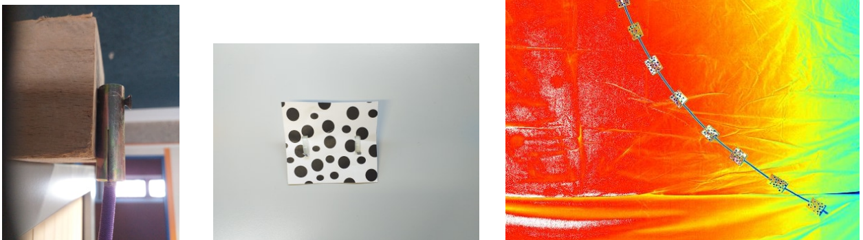
Figure 3.10: Hinge and target used for the experiment - Cable with targets mounted on
