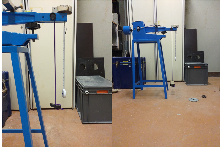
Figure 3.8: Extension of a linear elastic cable-type material
