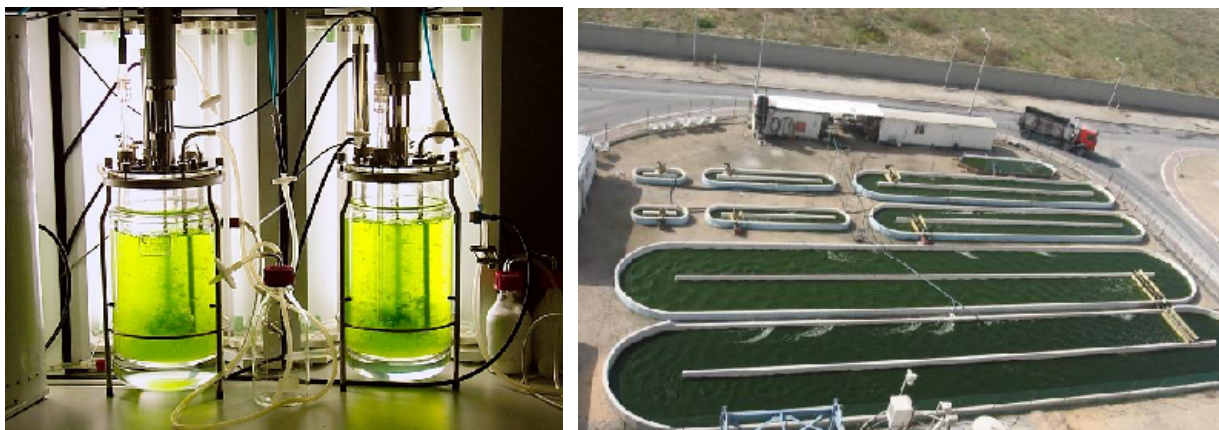
Figure 6.1: Typical setups for the culture of photosynthetic micro-organisms. Left A photo-bioreactor for moss culture (Freiburg University). Right An open raceway pond
