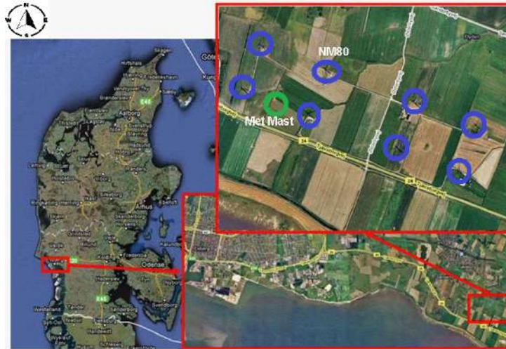
Figure 3.1 – Tjaereborg wind farm, the instrumented wind turbine is shown along with the other wind turbines. The met mast is also shown south-west to the instrumented turbine [148]. The wind turbines are circled in blue and the met mast in green.
