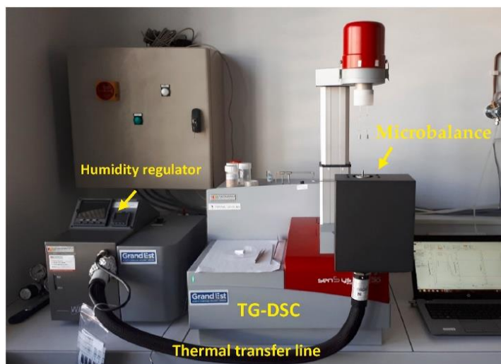
Figure 15. TG-DSC apparatus with a microbalance connected to a humidity generator (Wetsys) through a thermal transfer line (Setaram).
