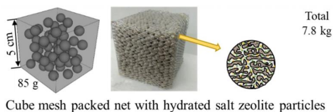
Figure 9. Representation of the Al cube mesh of 5 cm edge [20].
