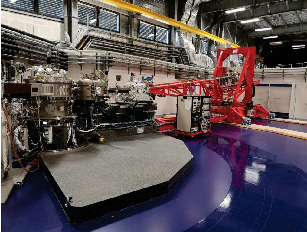
Figure V-2 Picture of the ID32 RIXS beamline setup
