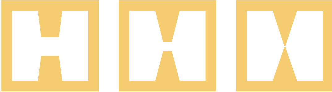
Figure 2.10: SRRs with identical \frac{A}{C} ratio, but decreasing confinement volume.
