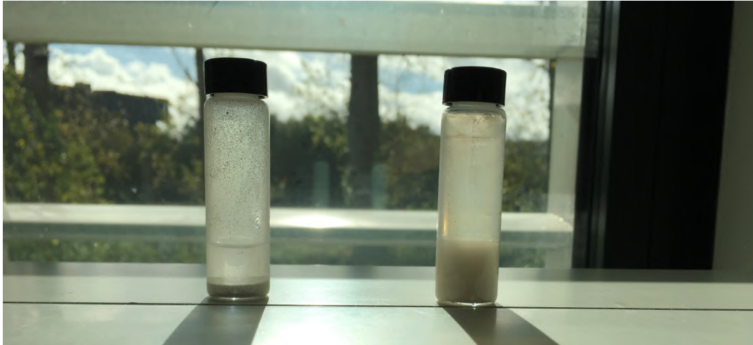
Figure 5.13: Photograph of diamond microparticles (sizes ranging from 0.5\ \mu\text{m} to 1\ \mu\text{m} ) in hexane. Left: Without surface treatment. Right: With OTS surface treatment. Both solutions were agitated a few seconds before the photograph was taken.
