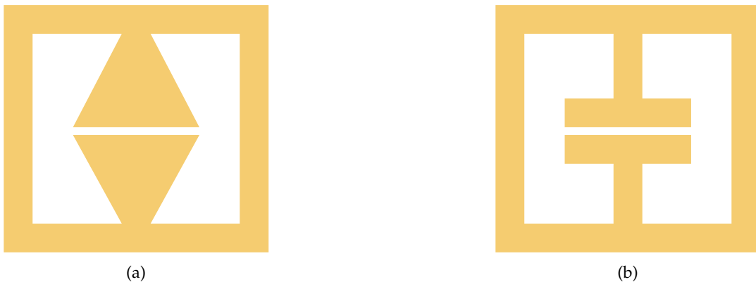
Figure 2.7: Two designs for SRR with large capacitance.
