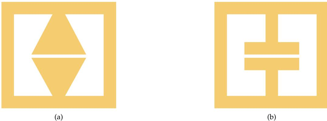
Figure 2.7: Two designs for SRR with large capacitance.
