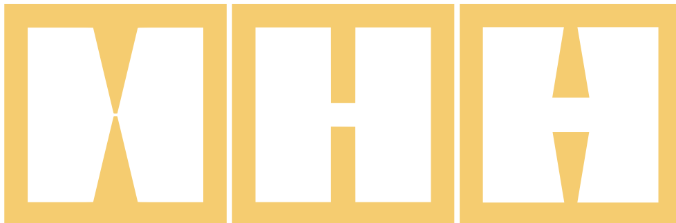
Figure 5.3: Example of electric split ring resonator designs with three different gap sizes ( 0.5\ \mu\text{m} , 4\ \mu\text{m} and 6\ \mu\text{m} ), the trapezoidal shape makes the capacitance independent of the gap size.
