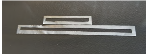
Figure 3.32: The loop resonators used for the measurement. The first resonator has g = 2 mm, w = 1.4 mm and l_1 = 47.97 mm. The second resonator has the same g and w but l_2 = 97 mm.
