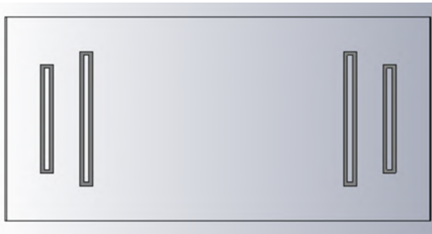
Figure 3.74: Set of 2 \times 2 loops working at different frequencies to achieve a distance sensing.
