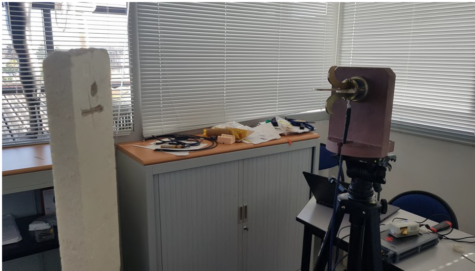
Figure 3.18: Test bench configuration for the mono-static measurement in an office.
