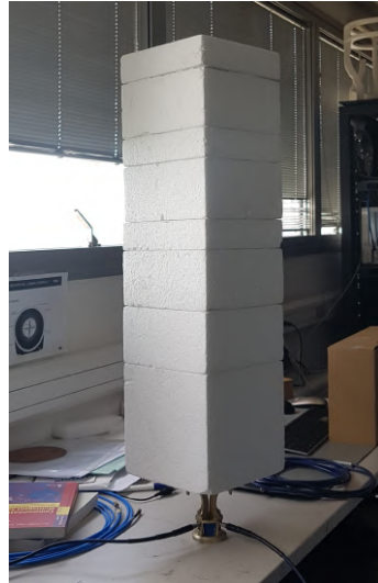
Figure 3.59: Measurement setup used to study the readable distance of the resonator.
