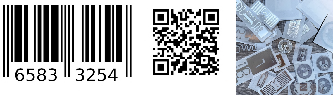
Figure 1.6: Identification technologies : a) 1D barcode (EAN 8), b) 2D barcode (QRcode), c) RFID tags.
