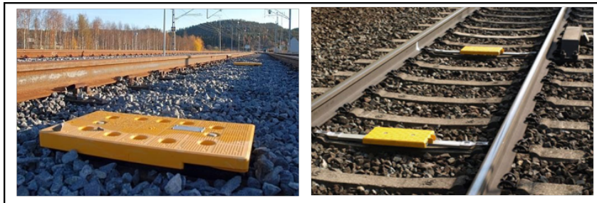
Figure 2.14: Physical Balises (PB) and Balise Groupe (BG)
