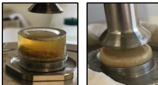
Figure 2.3 Left) The glass ring, posed on the lower geometry plate of the rheometer, was used as a container for the piece of gel and digestive juice; during the digestive juice infusion to the sample the temperature of the plate was set to 4°C. Right) the gel sample after the infusion time, before lowering the upper geometry plate and starting the digestion measurements in situ ; during the measurements, the temperature was set to 37°C and the temperature bonnet was covering the sample setup.
