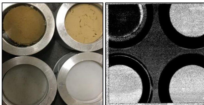
Figure 5.2 Left) Images of 4 different protein gels (100g/L) in circular cells ( \varnothing 40 mm); top - canola gels, bottom left- potato, bottom right - milk. Right) Corresponding Dark Field Images measured at the same gratings distance (corresponding to one value of q ).
