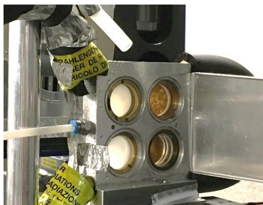
Figure 2.6 Image of the gel samples in neutron cells before the measurements. The metal cover was closed for the measurements time, to providing a better thermal control and avoiding condensation when submitted to the air jets.
