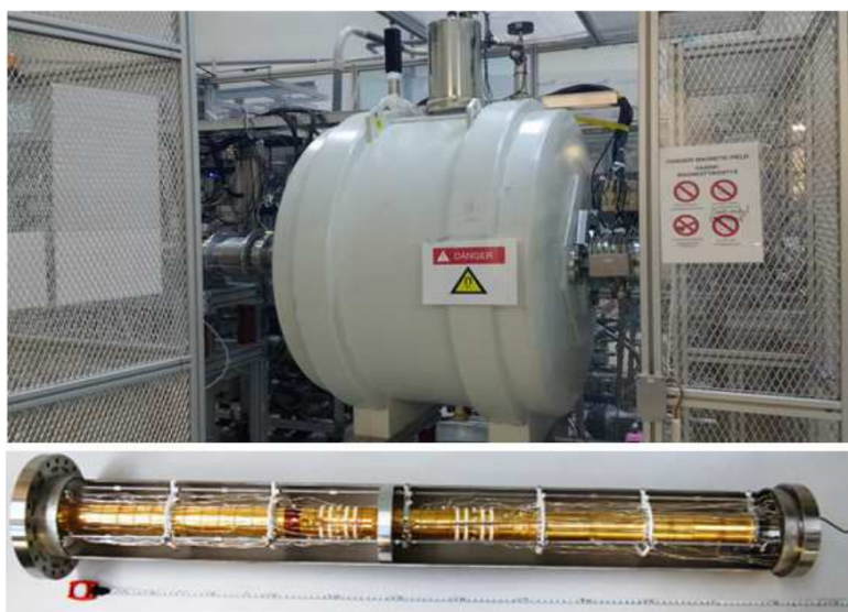
Figure 4.10: Top: The JYFLTRAP Penning trap superconducting magnet. Bottom: The gold-plated electrodes of the JYFLTRAP [101]
