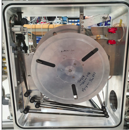
Figure 4.13: The IGISOL tape station as seen from the inside.
