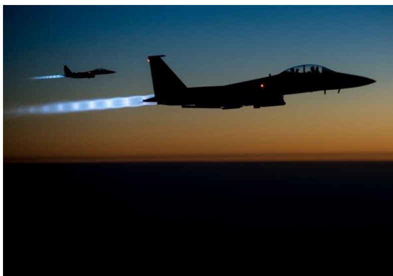
Figure II-11. Shock diamonds formed in the after body of an F-15 Fighter jet (Reuters)
