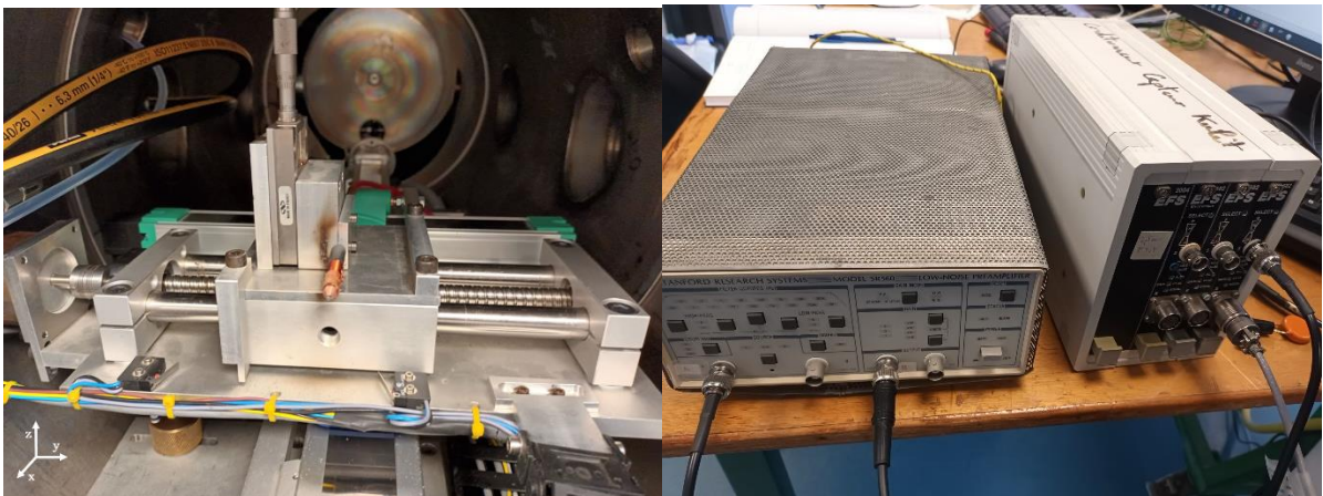
Figure VI-9. Left figure gives a frontal view in the direction of the flow of the rapid pressure sensor, right figure shows amplifier-filter and the Kulite conditioner (left to right), the filter has been used to filter the high frequency with a 3 KHz low pass filter.
