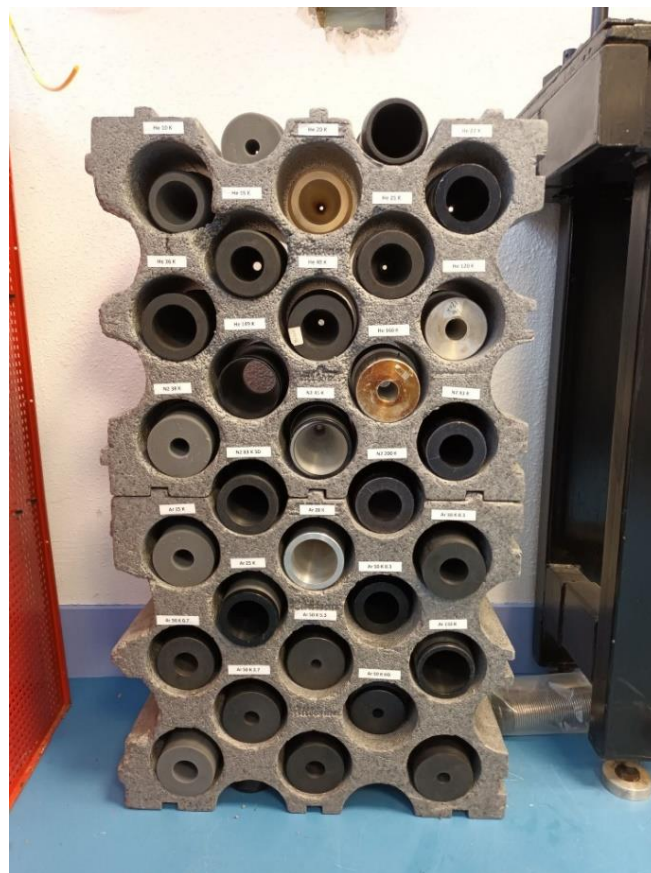
Figure III-6. Series of Laval nozzles used in Rennes, all the 3D printed nozzles have been designed and machined in this work 1 (All 3D printed nozzles used for this work and of colleagues are given in the Table of nozzles. See appendix A.III)
