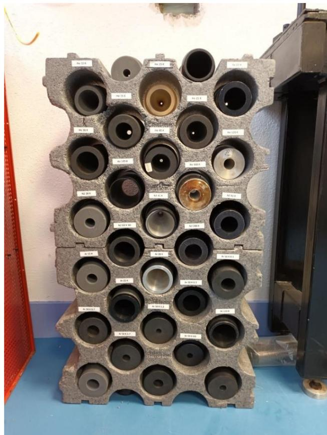
Figure III-6. Series of Laval nozzles used in Rennes, all the 3D printed nozzles have been designed and machined in this work<sup>1</sup> (All 3D printed nozzles used for this work and of colleagues are given in the Table of nozzles. See appendix A.III)
