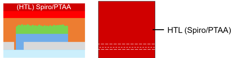
Figure 2.11: Side and top representation of substrates after HTL spin-coating.
