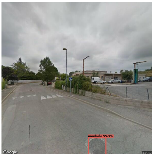
Figure 12 Example of manhole covers' detection using Google Street View images.
