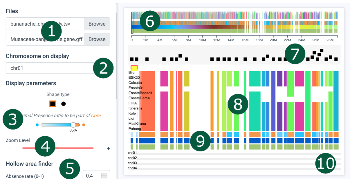
Figure 26: Panache’s UI is divided between a main view and a menu panel; The menu contains multiple interactive elements: 1) File loaders; 2) Choice of Panchromosome to display; 3) Core threshold; 4) Geometric zoom level; 5) The Hollow Area Finder (see Panache II.A.4); ...all of which dynamically update the main view composed of: 6) A miniature overview of the whole PAV matrix; 7) A beeswarm plot of gene annotations; 8) The PAV matrix displayed as panBlocks; 9) Tracks summarizing panBlocks; 10) Similar panBlocks across panchromosomes, when available.
