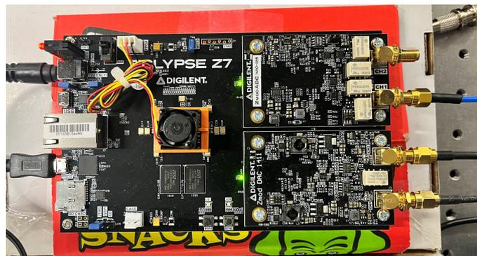
Figure 5.2: The image of our Eclipse Z7 FPGA board mounted with the dual-channel data converters (ADC and DAC).
