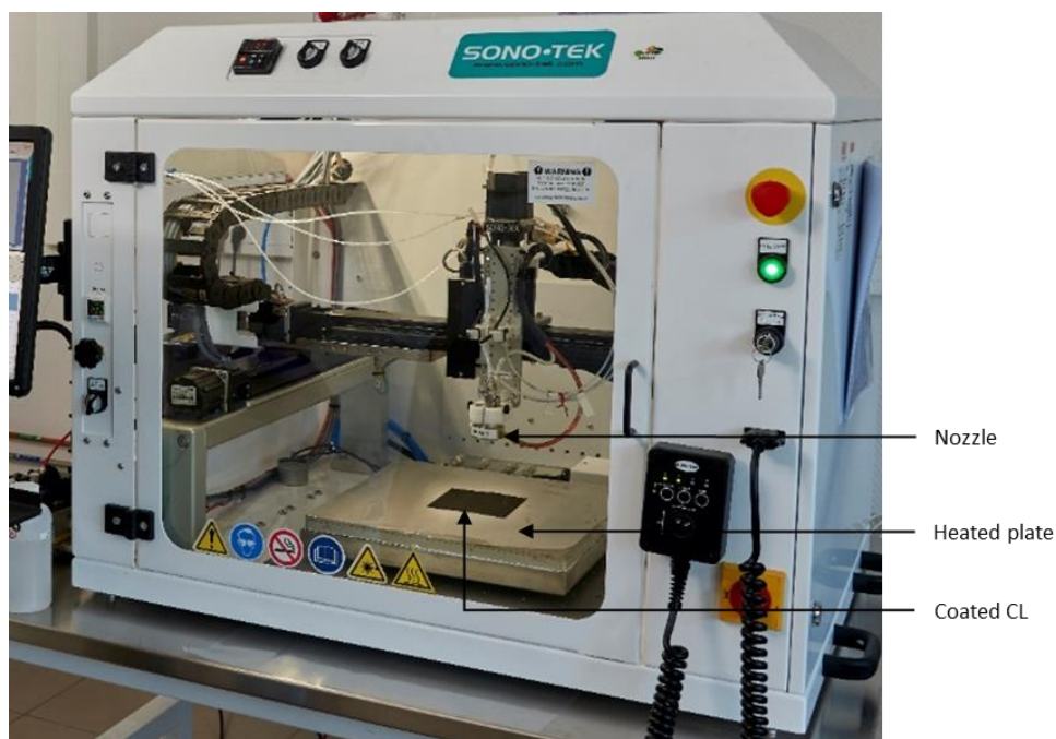
Figure II-7 : Picture of the Sono-tek machine used for spray coating method.
