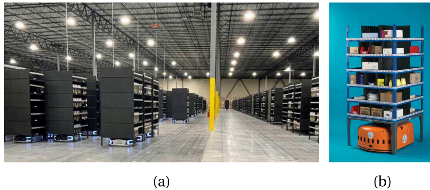
Figure 2.5: Exemple of robots used in warehouses for RMFS. (a) Warehouse using the Geek+™ solution and (b) Kiva robot carrying an inventory pod (source)
