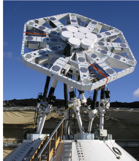
(b) The YTLA/AMiBA telescope on Mauna Loa in Hawaii lies on an hexapod mount [HAC+09].
