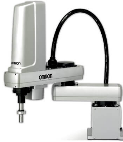
(b) A SCARA robot by Omron with four degrees of freedom: the end-effector can move in space in three directions and rotate about the vertical axis.
