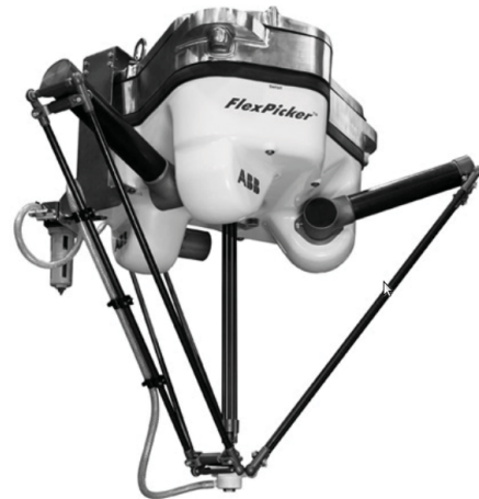
(b) The ABB FlexPicker DELTA robot.
