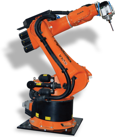
(a) A robotic arm with six degrees-of-freedom by Kuka. The robot tool can move and rotate in any direction in its workspace.
