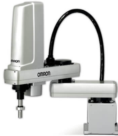
(b) A SCARA robot by Omicron with four degrees of freedom: the end-effector can move in space in three directions and rotate about the vertical axis.
