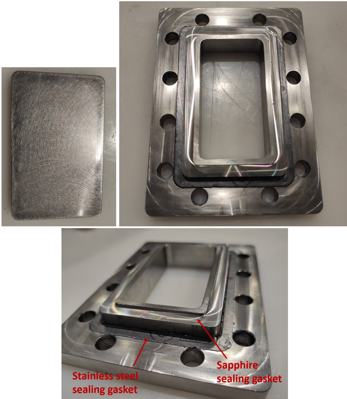
Figure 7.15: Stainless steel plate to replace broken window and the flange remanufactured with gasket grooves to ensure sealing at the test section body and sapphire levels.
