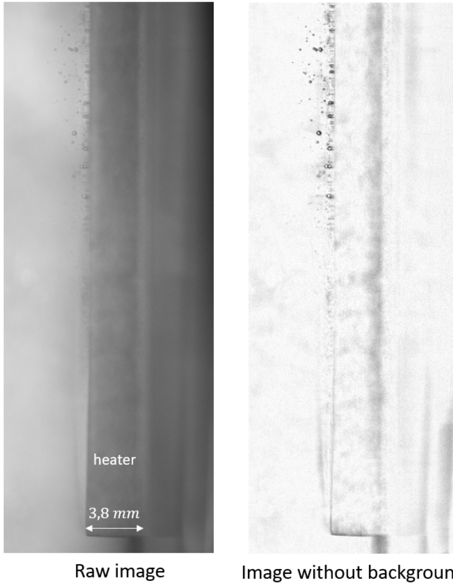
Figure 7.24: Example of a full frame image 2048 \times 1952 \text{ pxl} with 6600 \text{ i/s} record for: P = 120 \text{ bar} , Q = 1.21 \text{ m}^3/\text{hr} , T_{in} = 321^\circ\text{C} corresponding to a subcooling of \Delta T_{sub} = 3.7^\circ\text{C} . Raw image (left) and image without background (right).
