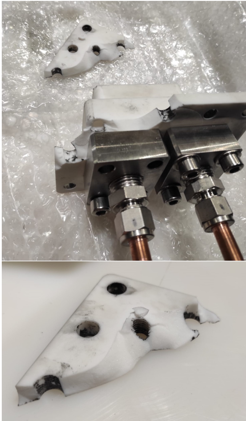
Figure 7.8: Breakage of the MACOR when assembling the plates, crack observed as soon as the first screw was tightened, when disassembling a breakage was observed with the threaded MACOR.
