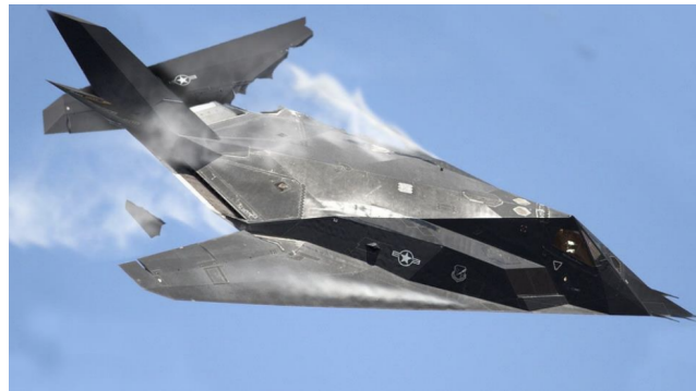
FIGURE 1.4: Failure of F-117 aircraft due to flutter [22].
