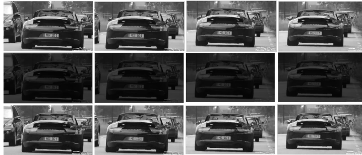
Figure 5.3: Example 2. First row: original frames. Second row: Blurred frames. Third row: Restored frames.
