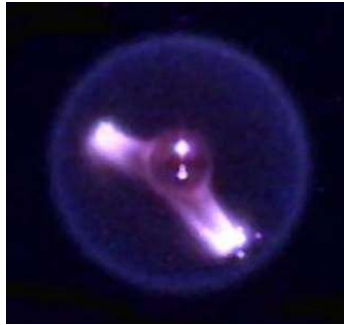
Figure I.1. Burning n -heptane droplet in the FLEX apparatus, image from [31].
