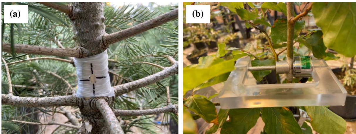
Figure 57. Installation steps of a stem psychrometer.
