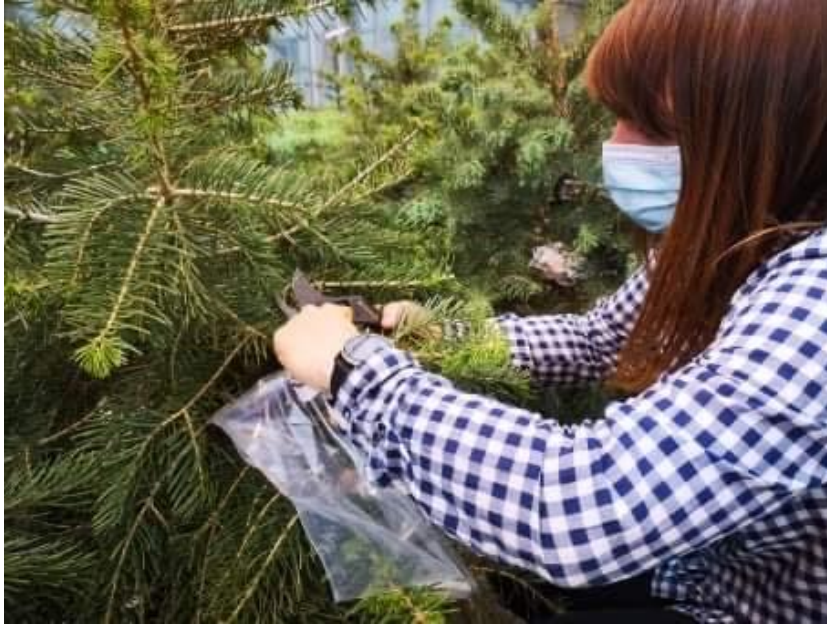
Figure 55. Sampling of branches nearby the LVDT sensor for physiological measurements. Branches were immediately stored in plastic bag to prevent further dehydration during transport between the glasshouse and the laboratory.
