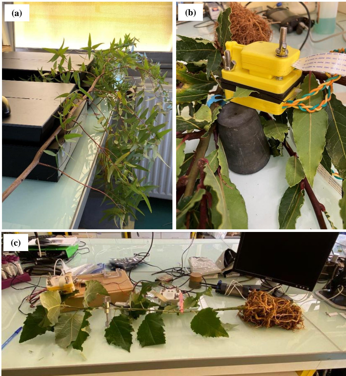
Figure 41. Plant bench dehydration and installation of the optical method. A. Eucalyptus viminalis tree installed on a scanner. B. Clamp with a camera installed on Laurus nobilis leaf. C. Bench dehydration of a Populus tremula x alba sapling equipped with a camera.
