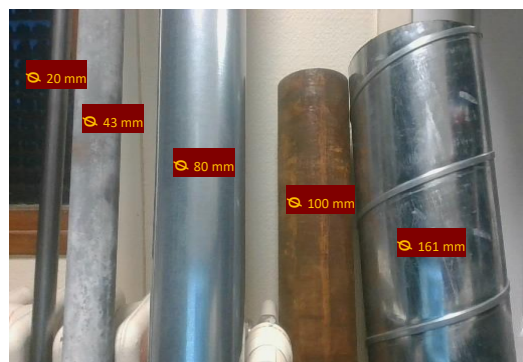
Figure 4.15: Metallic pipes used for experiment with its diameter size.
