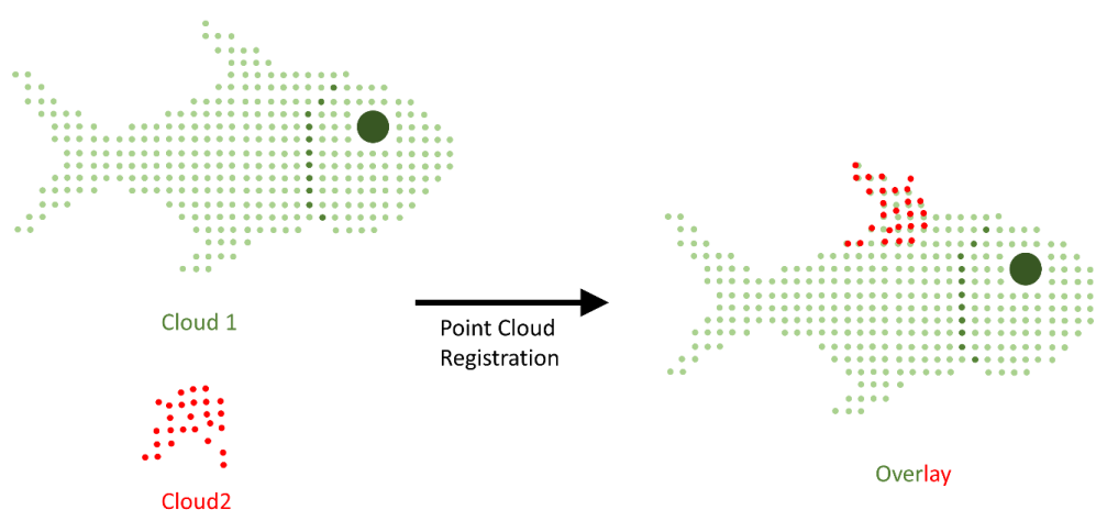
Figure 1. Schematic representation of point cloud registration. The red cloud is rotated and translated along its three main axes until the optimal alignment to the green cloud is found.
