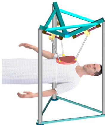
Figure II-11 : Robot 3-PRS
