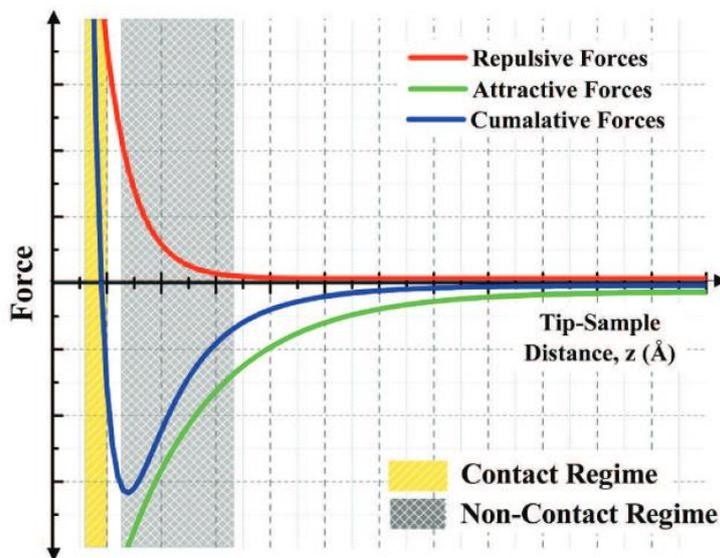
Figure 2. 7 : Force curve of an AFM tip as a function of surface distance. Extracted from<sup>93</sup>.
