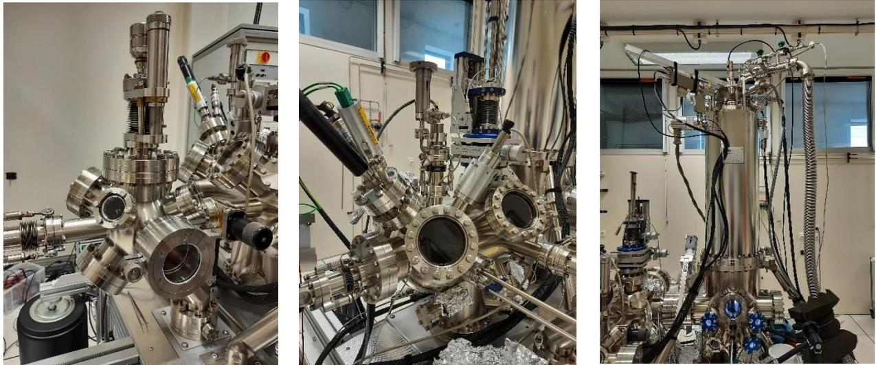
Figure 2. 13 : (left) Photo of the load lock side of the JT system (middle) photo of the preparation chamber of the JT system (right) Photo of the analysis chamber of the JT system.
