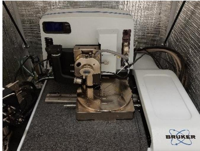
*Figure 2. 12: Photo of the Bruker ICON microscope.*
