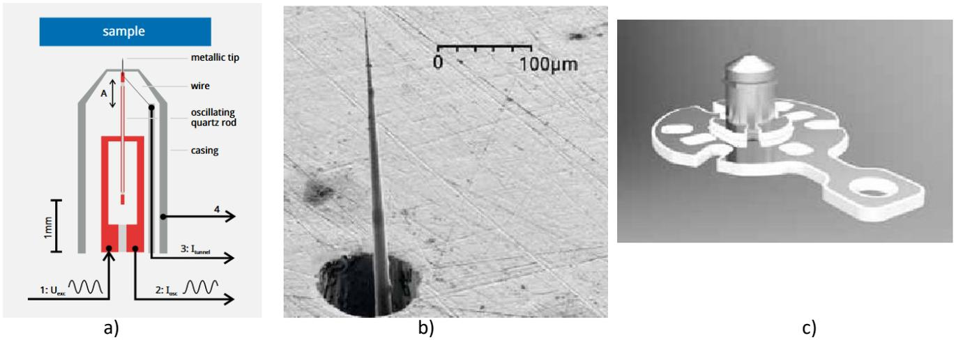
Figure 2. 11 : a) Schematic drawing of the KolibriSensor b) SEM image of Kolibri tip c) Handle plate of the KolibriSensor. Extracted from<sup>109</sup>.
