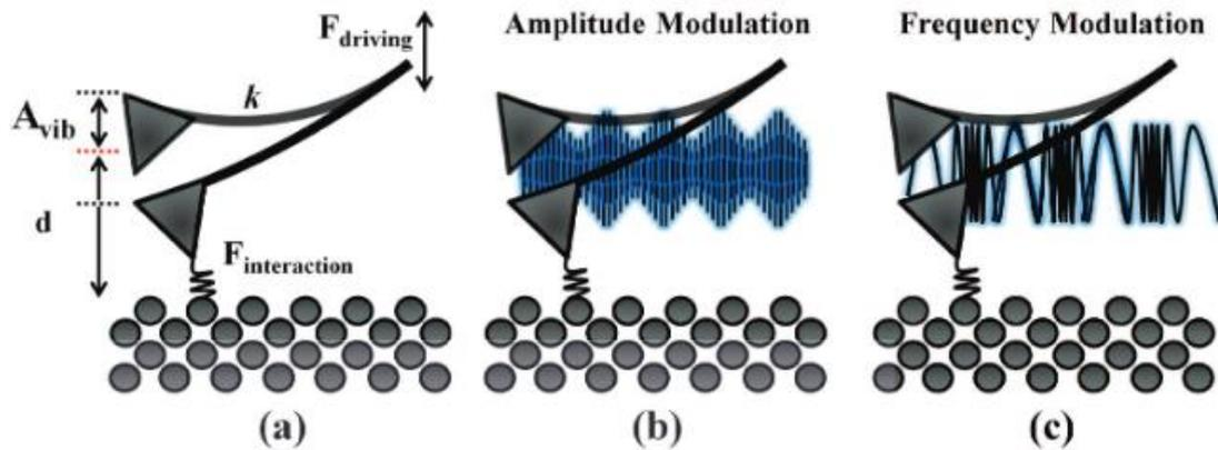
Figure 2. 4 : Driving force and tip-surface interaction force upon a vibrating cantilever (a) with a normal mode spring constant  $k$ , and with a vibrational amplitude,  $A_{vib}$ . Schematic representation of amplitude (b) and frequency modulation (c) AFM modes. Adapted from<sup>93</sup>.
