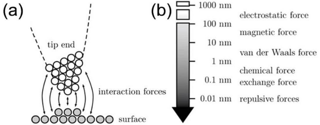
Figure 2. 5 : (a) Schematic representation of the tip-sample interaction forces (b) Representation of the forces that act at each z-scale. Adapted from<sup>93</sup>.
