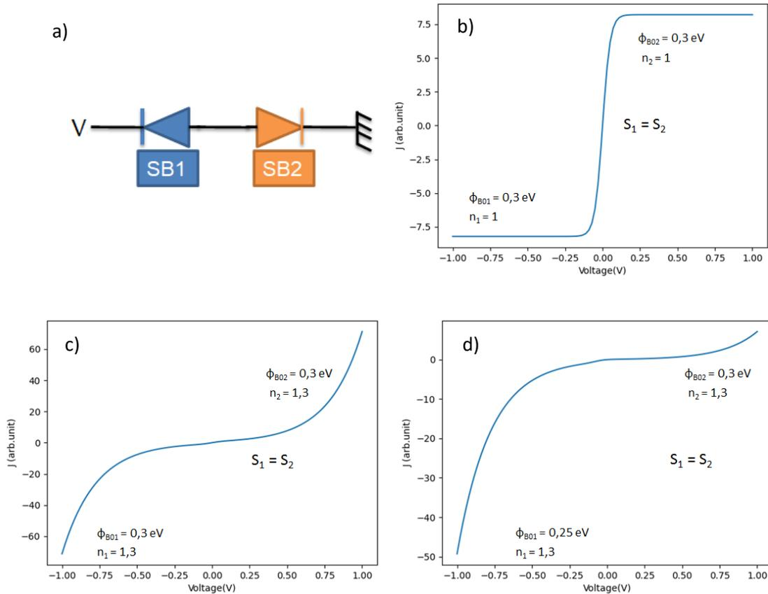
Figure 3. 9 : a) Equivalent circuit modeled by Eq. (3. 5). b) Simulated I-V characteristics for contact using  $\phi_{B01} = \phi_{B02} = 0.3 \text{ V}$ , the same junction area  $S_1 = S_2$ , and a perfect ideality factor ( $n=1$ ). c) Simulated characteristics, introducing an ideality factor  $n=1.3$ . c) Simulated I-V characteristic using asymmetric barrier heights  $\phi_{B01}=0.25 \text{ V}$ ,  $\phi_{B02} = 0.3 \text{ V}$ ,  $S_1 = S_2$ , and an ideality factor  $n=1.3$ .
