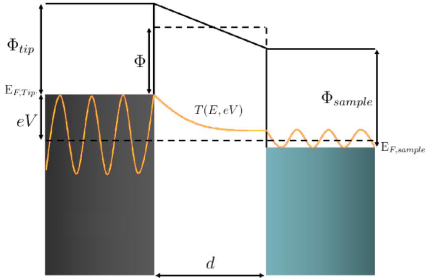
Figure 2. 2 : Schematic energy diagram of the tunnel junction in a STM. Adapted from<sup>94</sup>.
