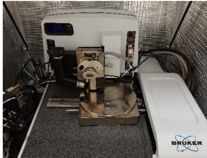
Figure 2. 12: Photo of the Bruker ICON microscope.
